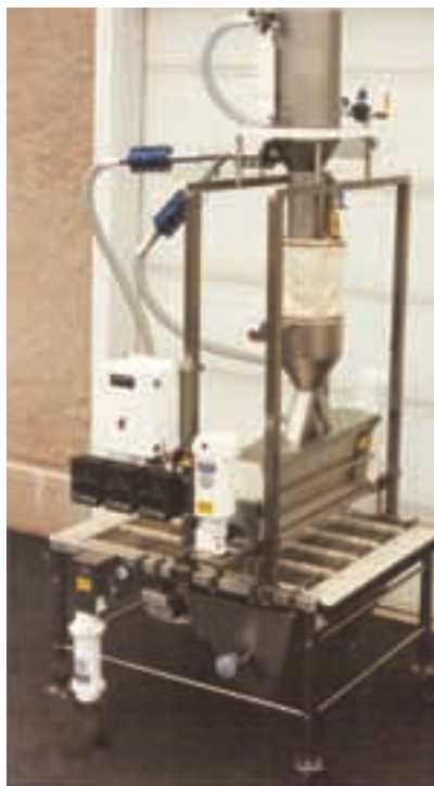
▲ A vacuum fill system is mounted on top of this dry material dispenser, which features a mesh conveyor and a reclaim hopper.
